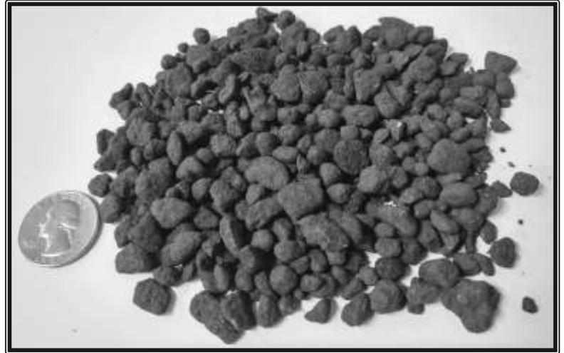
AquaGate+RemBind serves as a delivery mechanism to reliably and uniformly place reactive materials into aquatic and other challenging environments.
